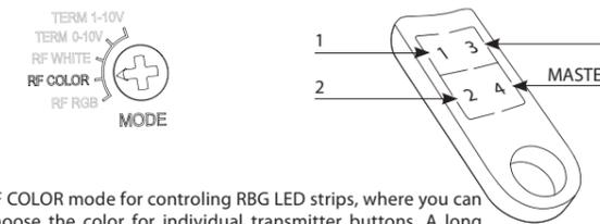
RF COLOR mode for controlling RGB LED strips, where you can choose the color for individual transmitter buttons. A long press of the button starts the color search mode. After releasing the button, the current color is set for the given button.
