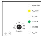
switching power supply works correctly output voltage 27V is correct (U<sub>OUT</sub>>24V) low output voltage 12V (short-circuit, overload) batteries are recharged
