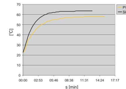
PVC - reaction to water temperature from 22.5 1°C to 58°C.
