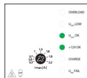
switching power supply not working correctly - UPS mode output voltage 27V is correct (U<sub>OUT</sub>>24V) output voltage 12V is correct batteries are not recharged
