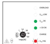
switching power supply works correctly output voltage 27V is correct (U<sub>OUT</sub>>24V) output voltage 12V is correct batteries are recharged
