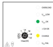
switching power supply is overload low output voltage 27V (U<sub>OUT</sub><21V) low output voltage 12V batteries are not recharged
