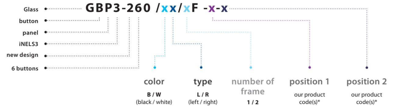
\* In case of 1-module choice it is necessary to pick 2x 1-module to fill up the 1 position, for example GBP3-260/WL/1F-21W45W.
