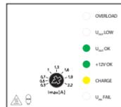
switching power supply not working correctly - UPS mode low output voltage 27V (21V<U<sub>OUT</sub><24V) output voltage 12V is correct batteries are not recharged
