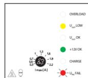
switching power supply works correctly low output voltage 27V (21V<U<sub>OUT</sub><24V) output voltage 12V is correct batteries are not recharged
