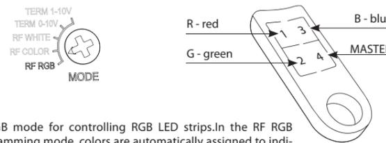
RF RGB mode for controlling RGB LED strips. In the RF RGB programming mode, colors are automatically assigned to individual transmitter buttons.
