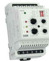
monitors overcurrent or undercurrent in AC or DC circuits in 3 ranges, 2x independent output contacts WINDOW
