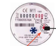
Rotating water meter indicator
