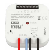
RFJA-32B Switch unit for shutters - 2x 8 A
