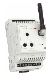
RFDEL-71M Universal dimmer, 1-channel - 1x 600 VA - R, L, C, LED, ESL
