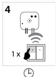
After the desired time has elapsed, the timing mode ends by pressing the button on the RF transmitter, to which the sunrise function is assigned. This stores the set time interval into the actuator memory.
