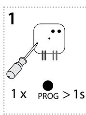
Press of programming button on actuator RFDEL-71B for 1 second will activate actuator RFDEL-71B into programming mode. LED is flashing in 1s interval.
