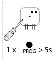
Bypassing the programming button on the actuator for 5 seconds, deletion of one transmitter activates. LED flashes 4x in each 1s interval.
