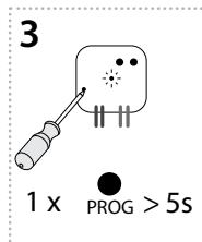
Press of programming button longer than 5 seconds, will activate actuator into timing mode. LED flashes 2x in each 1s interval. After releasing the button, the time of the sunset function begins to count down (period of complete dimming of the light).
