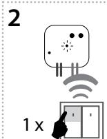
A press of your selected button on the RF transmitter assigns the function light scene 1.
