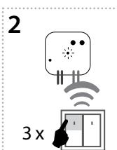
Three presses of your selected button on the RF transmitter assigns the function light scene 3 (must be a lapse of 1s between individual presses).
