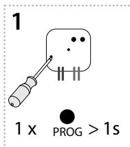
Press of programming button on receiver RFDEL-71B for 1 second will activate receiver RFDEL-71B into programming mode. LED is flashing in 1s interval.
