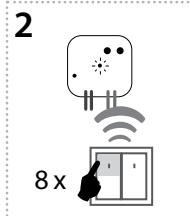
Eight presses of selected button on the RF transmitter assigns the function OFF (must be a lapse of 1s between individual presses).
