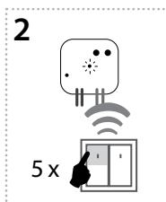
Assignment of the sunrise function is performed by five presses of the selected button on the RF transmitter (must be a lapse of 1s between individual presses).
