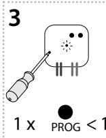
Press of programming button on actuator RFDEL-71B shorter than 1 second will finish programming mode. The LED lights up according to the preset memory function.
