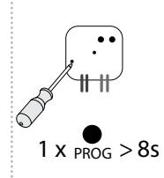
Bypassing the programming button on the actuator for 8 seconds, deletion occurs of the actuator's entire memory. LED flashes 4x in each 1s interval.
