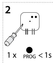
Pressing the programming button on the RFDEL-71B receiver for less than 1 second will finish the programming mode, this will reverse the memory function. The LED lights up according to the current pre-set memory function. The set memory function is saved.
