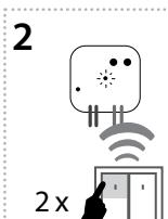
Two presses of your selected button on the RF transmitter assigns the function light scene 2 (must be a lapse of 1s between individual presses).
