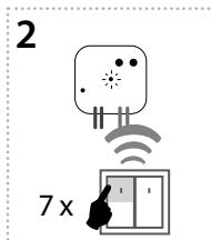
Seven presses of your selected button on the RF transmitter assigns the function ON/OFF (must be a lapse of 1s between individual presses).
