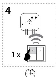
After the desired time has elapsed, the timing mode ends by pressing the button on the RF transmitter, to which the sunset function is assigned. This stores the set time interval into the actuator memory.
