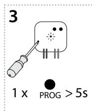
Press of programming button longer than 5 seconds, will activate actuator into timing mode. LED flashes 2x in each 1s interval. After releasing the button, the time of the sunrise function begins to count down (period of complete illumination of the light).
