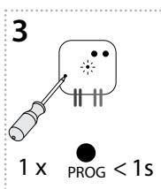
Press of programming button on actuator RFDEL-71B shorter than 1 second will finish programming mode. The LED lights up according to the pre-set memory function.
