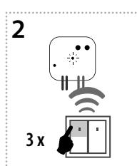
Three presses of your selected button on the RF transmitter assigns the function light scene 3 (must be a lapse of 1s between individual presses).
