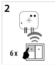
Assignment of the sunset function is performed by six presses of the selected button on the RF transmitter (must be a lapse of 1s between individual presses).
