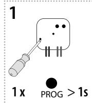
Press of programming button on actuator RFDEL-71B for 1 second will activate actuator RFDEL-71B into programming mode. LED is flashing in 1s interval.
