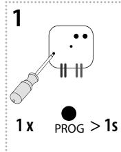
Press of programming button on actuator RFDEL-71B for 1 second will activate actuator RFDEL-71B into programming mode. LED is flashing in 1s interval.
