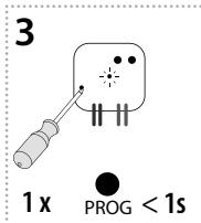
Press of programming button on actuator RFDEL-71B shorter than 1 second will finish programming mode. The LED lights up according to the pre-set memory function.
