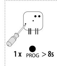
By pressing the programming button on the actuator for 8 seconds, deletion occurs of the actuator's entire memory. LED flashes 4x in each 1s interval. The actuator goes into the programming mode, the LED flashes in 0.5s intervals (max. 4 min). You can return to the operating mode by pressing the Prog button for less than 1s. The LED lights up according to the pre-set memory function and the component returns to the operating mode. Deletion does not affect the pre-set memory function.
