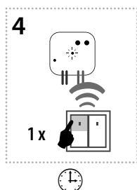
After the desired time has elapsed, the timing mode ends by pressing the button on the RF transmitter, to which the sunrise function is assigned. This stores the set time interval into the actuator memory.
