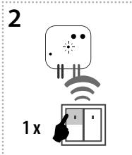
A press of your selected button on the RF transmitter assigns the function light scene 1.
