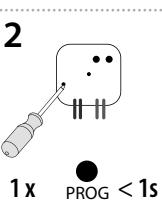
Pressing the programming button on the RFDEL-71B receiver for less than 1 second will finish the programming mode, this will reverse the memory function. The LED lights up according to the current pre-set memory function. The set memory function is saved.
