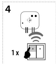
After the desired time has elapsed, the timing mode ends by pressing the button on the RF transmitter, to which the sunset function is assigned. This stores the set time interval into the actuator memory.
