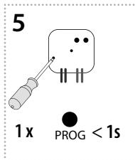
Press of programming button on actuator RFDEL-71B shorter then 1 second will finish programming mode. The LED lights up according to the pre-set memory function.
