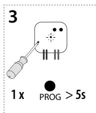
Press of programming button longer than 5 seconds, will activate actuator into timing mode. LED flashes 2x in each 1s interval. After releasing the button, the time of the sunrise function begins to count down (period of complete illumination of the light).
