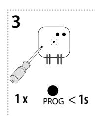
Press of programming button on actuator RFDEL-71B shorter than 1 second will finish programming mode. The LED lights up according to the pre-set memory function.
