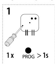
Press of programming button on actuator RFDEL-71B for 1 second will activate actuator RFDEL-71B into programming mode. LED is flashing in 1s interval.
