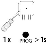
Press of programming button on receiver RFSA-x1B for 1 second will activate receiver RFSA-x1B into programming mode. LED is flashing in 1s interval.
