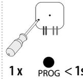
Pressing the programming button on the RFSA-x1B receiver for less than 1 second will finish the programming mode, this will reverse the memory function. The LED lights up according to the current pre-set memory function. The set memory function is saved.
