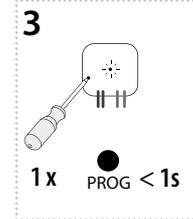
Press of programming button on actuator RFSA-11B shorter than 1 second will finish programming mode. The LED lights up according to the pre-set memory function.
