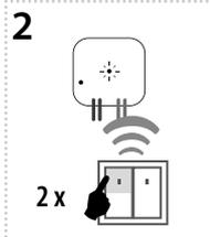
Two presses of your selected button on the RF transmitter assigns the function switch on (must be a lapse of 1 s between individual presses).
