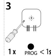
Press of programming button on actuator RFSA-61B shorter than 1 second will finish programming mode. The LED lights up according to the pre-set memory function.
