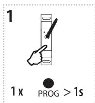
Press of programming button on receiver RFSA-61M/MI (66M/MI) for 1 second will activate receiver RFSA-61M/MI (66M/MI) into programming mode. LED is flashing in 1s interval.
