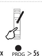
Press of programming button longer then 5 seconds, will activate actuator into timing mode. LED flashes 2x in each 1s interval. Upon releasing the button, the delayed return time starts counting.
