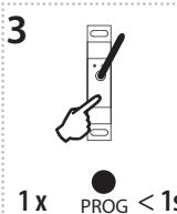
Press of programming button on receiver RFSA-61M/MI (66M/MI) shorter than 1 second will finish programming mode. The LED lights up according to the pre-set memory function.
