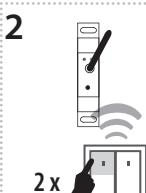
Two presses of your selected button on the RF transmitter assigns the function switch on (must be a lapse of 1s between individual presses).
