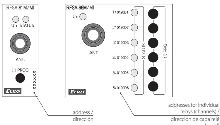
RFSA-61M/MI: the address listed on the front side of the actuator is used for programming and controlling an RF actuator by control units.
