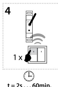
After the desired time has elapsed (range of 2s...60min), the timing mode ends by pressing the button on the RF transmitter, to which the delayed return function is assigned. This stores the set time interval into the actuator memory.
