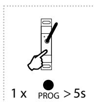
Bypressing the programming button on the actuator for 5 seconds, deletion of one transmitter activates. LED flashes 4x in each 1s interval.
