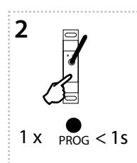
Pressing the programming button on the RFSA-61M(66M) receiver for less than 1 second will finish the programming mode, this will reverse the memory function. The LED lights up according to the current pre-set memory function. The set memory function is saved.
