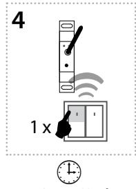
After the desired time has elapsed (range of 2s...60min), the timing mode ends by pressing the button on the RF transmitter, to which the delayed return function is assigned. This stores the set time interval into the actuator memory.
