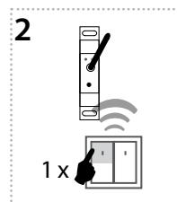
Select and press one button on wireless switch, to this button will be assigned function Button.
