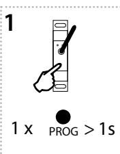
Press of programming button on receiver RFSA-61M (66M) for 1 second will activate receiver RFSA-61M (66M) into programming mode, LED is flashing in 1s interval.
