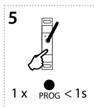
Press of programming button on receiver RFSA-61M (66M) shorter than 1 second will finish programming mode. The LED lights up according to the pre-set memory function.
