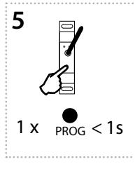
Press of programming button on receiver RFSA-61M (66M) shorter than 1 second will finish programming mode. The LED lights up according to the pre-set memory function.
