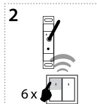
Assignment of the delayed on function is performed by six presses of the selected button on the RF transmitter (must be a lapse of 1s between individual presses).
