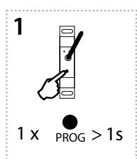
Press of programming button on receiver RFSA-61M (66M) for 1 second will activate receiver RFSA-61M (66M) into programming mode. LED is flashing in 1s interval.
