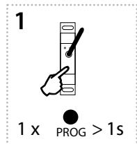
Press of programming button on receiver RFSA-61M (66M) for 1 second will activate receiver RFSA-61M (66M) into programming mode. LED is flashing in 1s interval.
