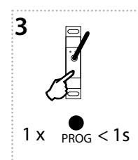
Press of programming button on receiver RFSA-61M (66M) shorter than 1 second will finish programming mode. The LED lights up according to the pre-set memory function.
