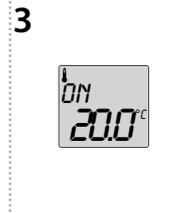
5 seconds after the last pressing of the button, the display of the set temperature switches back to the current temperature - the value is saved in the memory.
