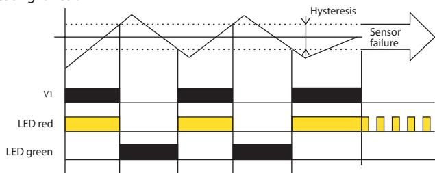
TEV-2 and TEV-3 are universal single thermostats for universal use. In case ambient temperature is higher than set temperature relay is open (function HEATING). For cooling function (opposite function) is possible to use NC contact of relay (V2).
